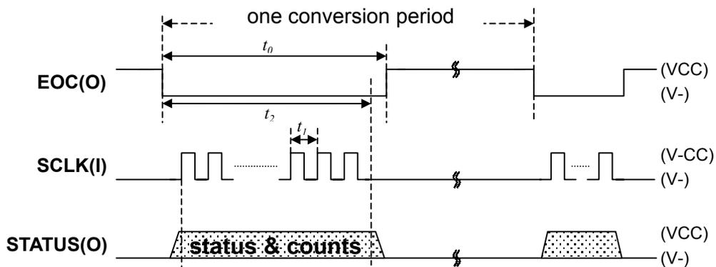
$t_0$  is at least 5ms and  $t_1$  must be  $(32 \sim 512)T$ , where  $T = 0.25\mu s$ .
