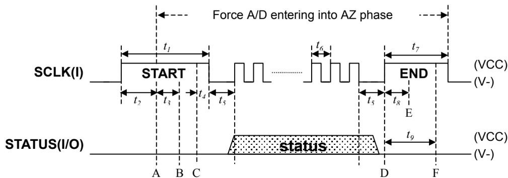
Timing of the above figure:  $(T = 0.25\mu\text{s})$
