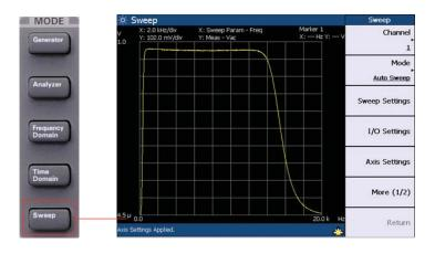
Figure 5: Use a single button to access the swept measurement mode.
