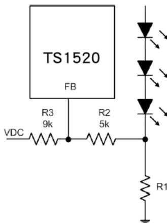
Figure 1. Dimming Control Using a DC Voltage
