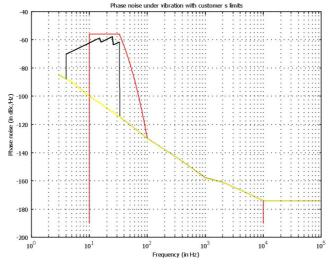
Figure 2 : Phase noise curves @ 100 MHz
