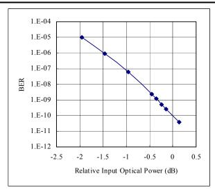
The figure shows the relationship between typical trade-off of BER and Relative Input Optical Power. Besides the required BER =  $1 \times 10^{-10}$  of the ATM Forum 155.52 Mbps Physical Layer Standard, The transceiver can be operated at other Bit-Error-Rate conditions. The Relative Input Optical Power in dB is referenced to the actual sensitivity of the device. For BER conditions better than  $1 \times 10^{-10}$ , more input signal is needed (+dB).
