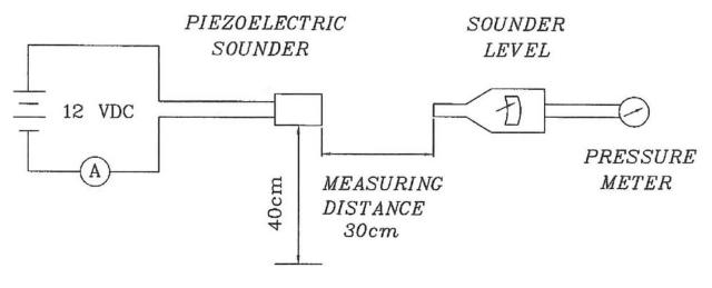
S.P.L. Measuring Circuit Mic: RION S.P.L. meter UC 30 or equivalent
