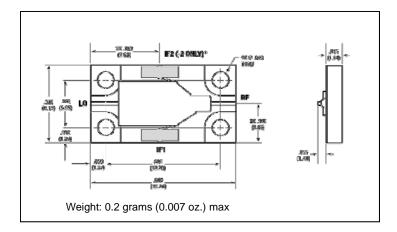
For base model, only the IF1 port is connected. For the "-2" model, only the IF2 port is connected.
