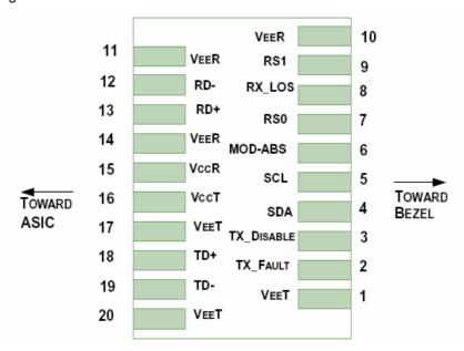
Figure 3, Host PCB Pinout Top View
