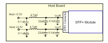
Figure 1, Recommended Host Board Power Supply Circuit
