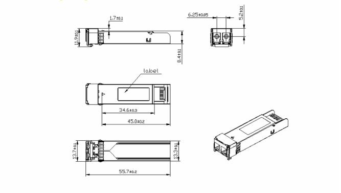
Figure 4, Mechanical Design Diagram of SFP+
