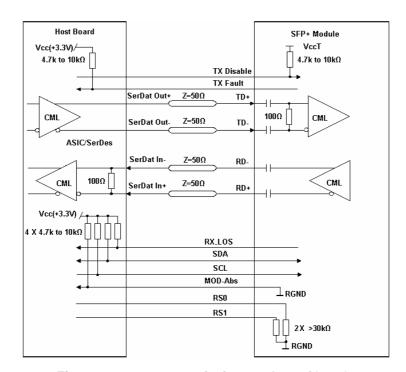
Figure 2, Recommended Interface Circuit
