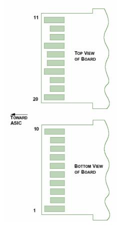
Figure 4, SFP+ module PCB Pinout Fiberxon Proprietary and Confidential, Do Not Copy or Distribute
