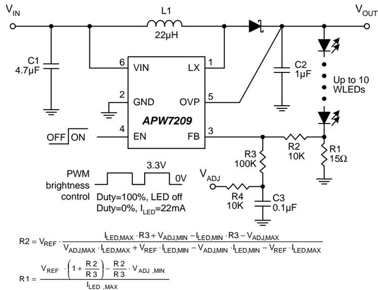
Figure 3. Brightness control using a filtered PWM signal
