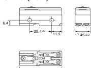
Note: 1. Appropriate terminal screw tightening torque: 0.78 to 1.18 N·m.
