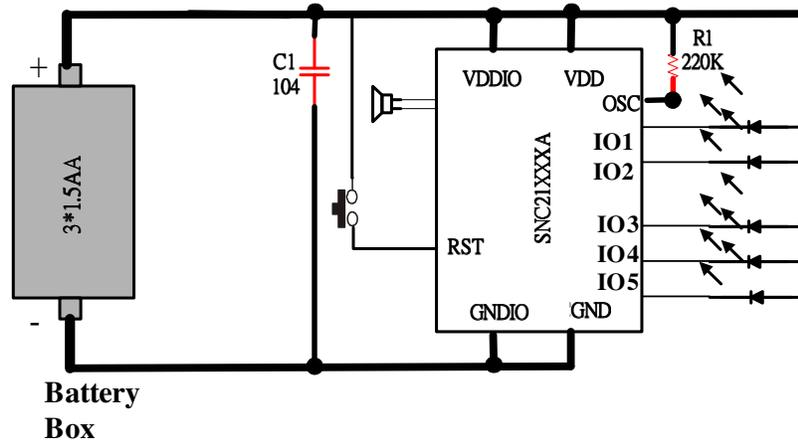
It is suggested to add a capacitor (C1), 104, between VDD with GND to keep power stable with general application. And this capacitor is strongly suggested to be as close to the chip as possible.
