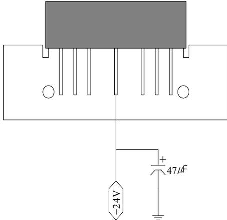
1. On the power input port (Pin#5), 47µF/35V capacitor GND is recommended.
