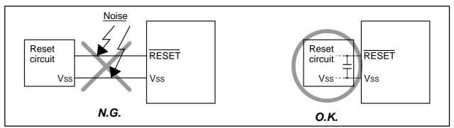
Figure 1.1.2. Wiring for RESET pin
