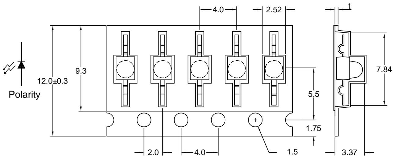
Note : The tolerances unless mentioned is  $\pm 0.2$ mm, Angle  $\pm 0.5$ . Unit=mm.
