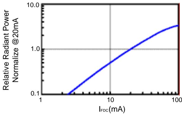
Fig.4 Relative Radiant Power vs. Forward Peak Current
