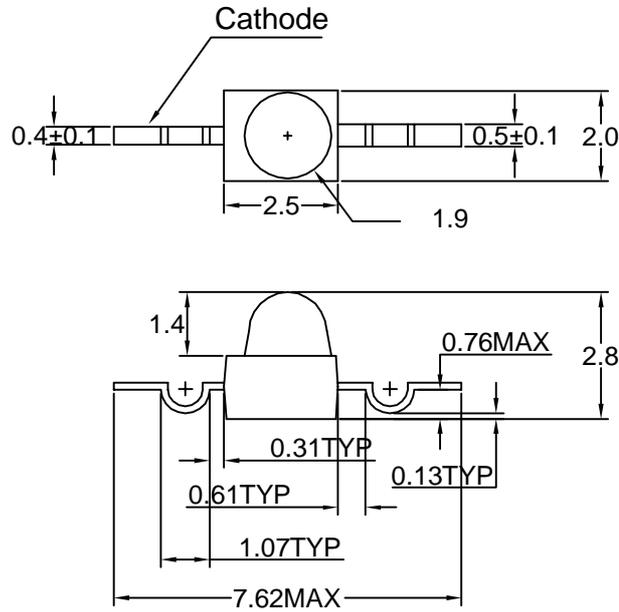
Note : 1.All dimension are in millimeter tolerance is  $\pm 0.2$ mm unless otherwise noted.
