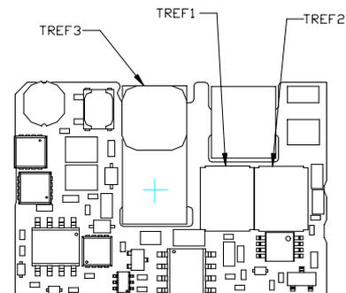
**Figure 13.  $T_{ref}$  Temperature Measurement Locations.**
