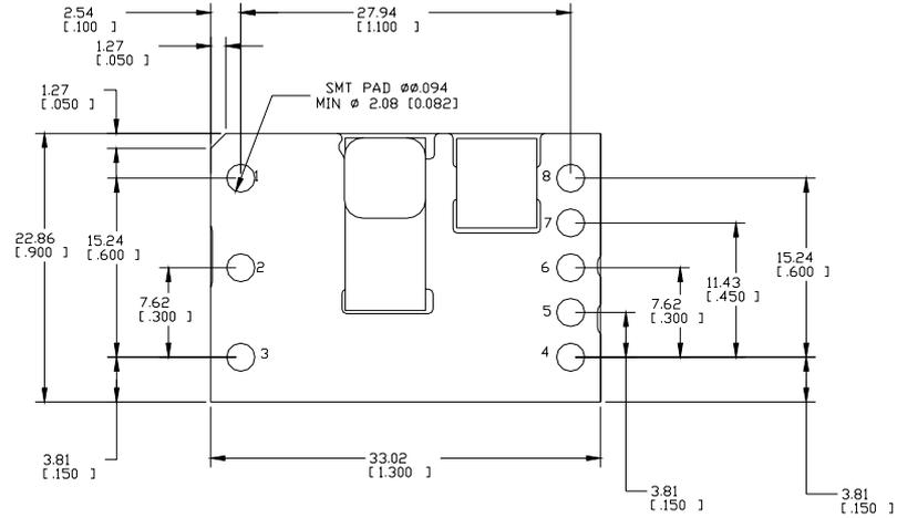
SMT Recommended Pad Layout (Component Side View)
