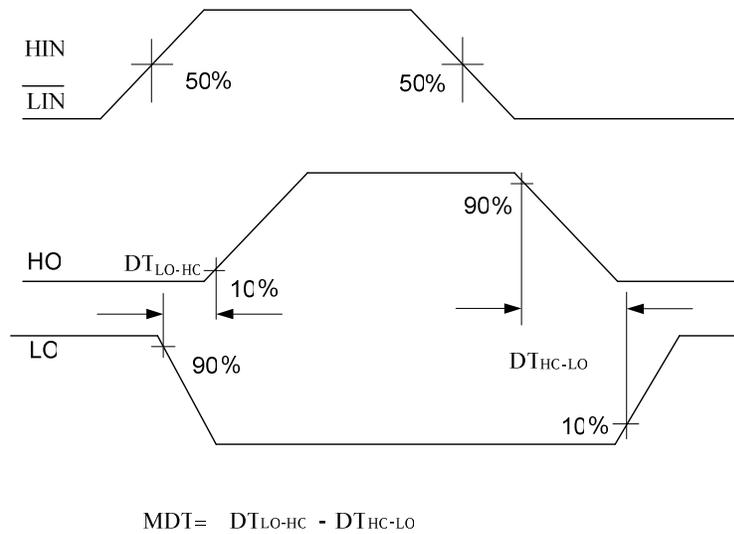
**Figure 5: Delay Matching Waveform Definition**
