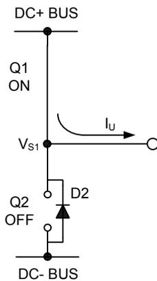
**Figure 11: Q1 conducting**
