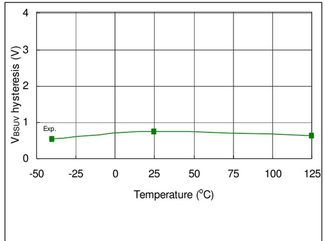
Fig. 27. V<sub>BS</sub> Supply UV Hysteresis vs. Temperature
