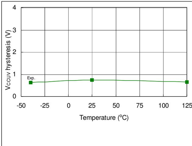
Fig. 26. V<sub>CC</sub> Supply UV Hysteresis vs. Temperature
