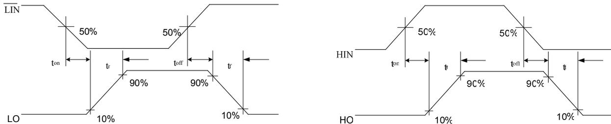
**Figure 3: Switching time waveforms**
