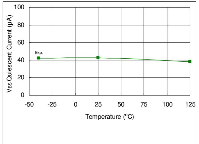
Fig. 29 V<sub>BS</sub> Quiescent Supply Current vs. Temperature
