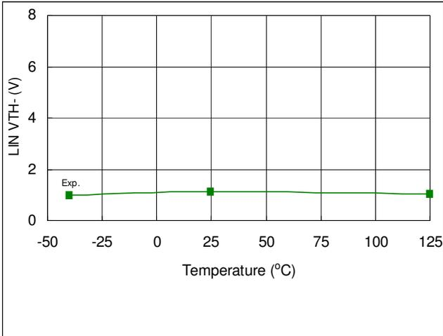
Fig. 38. LIN V<sub>TH-</sub> vs. Temperature
