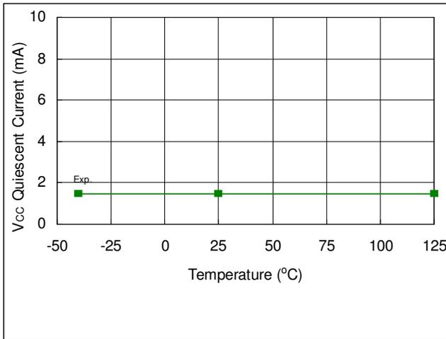
Fig. 28. V<sub>CC</sub> Quiescent Supply Current vs. Temperature
