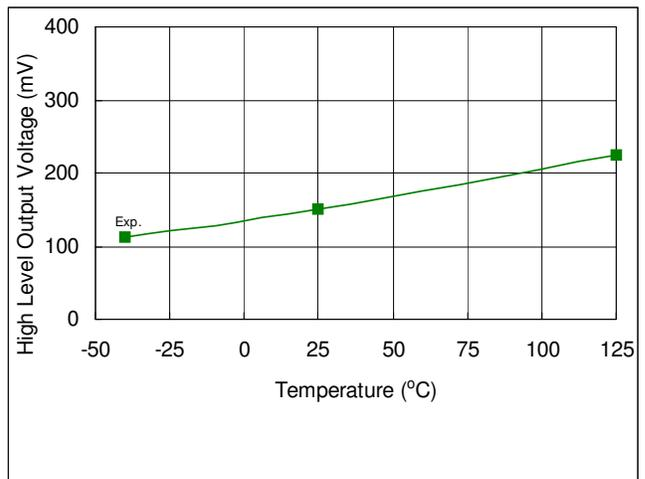
Fig. 35. High Level Output Voltage vs. Temperature
