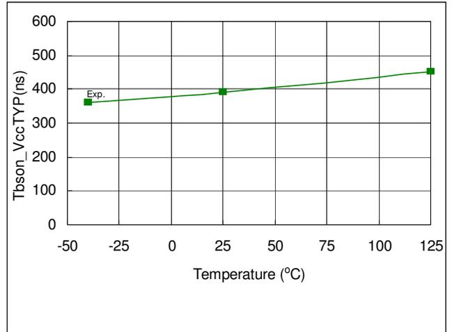
Fig. 41. T<sub>bson\_VccTYP</sub> vs. Temperature
