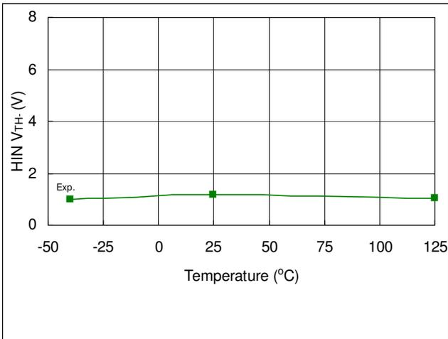
Fig. 40. HIN V<sub>TH-</sub> vs. Temperature
