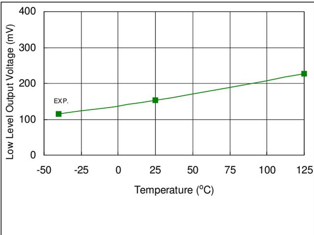
Fig. 34. Low Level Output Voltage vs. Temperature
