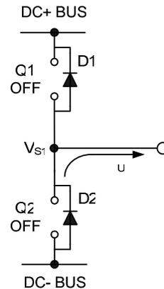
**Figure 12: D2 conducting**
