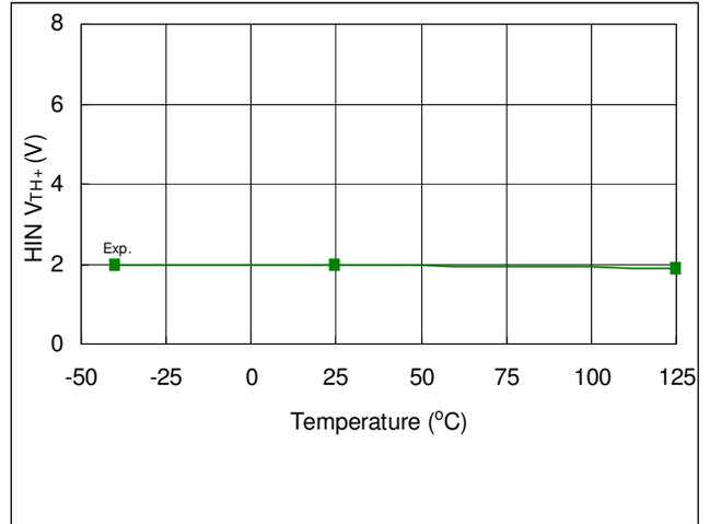
Fig. 39. HIN V<sub>TH+</sub> vs. Temperature
