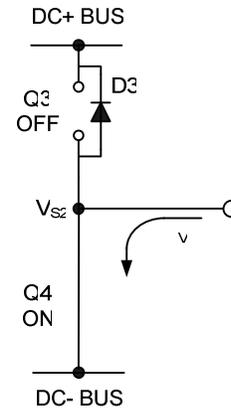
Figure 14: Q4 conducting
