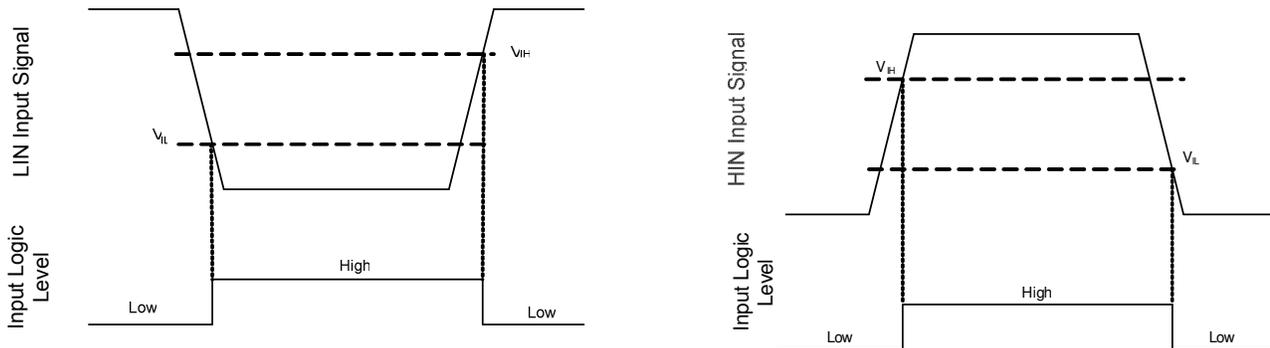
**Figure 6: HIN & LIN input thresholds**
