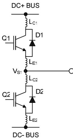
Figure 15: Parasitic Elements
