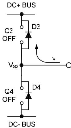
Figure 13: D3 conducting
