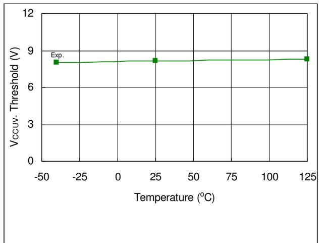
Fig. 31. V<sub>CCUV-</sub> Threshold vs. Temperature
