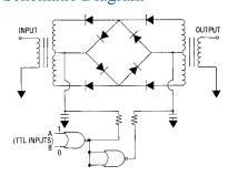
DC volts:  $5\pm1\%$  nominal; DC current 45 mA TTL logic inputs "0" = 0 volt
