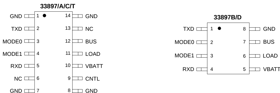
Figure 4. 33897/A/B/C/D/T Pin Connections
