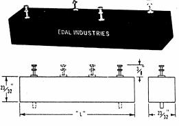
"L" is equal to ½ inch per KV plus 1½" for half wave circuit.
