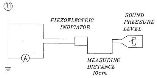
S.P.L. Measuring Circuit Mic: RION S.P.L. meter UC30 or equivalent
