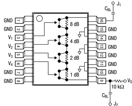
DC blocking capacitors ( $C_{BL}$ ) and biasing resistor must be supplied externally for positive voltage operation.
