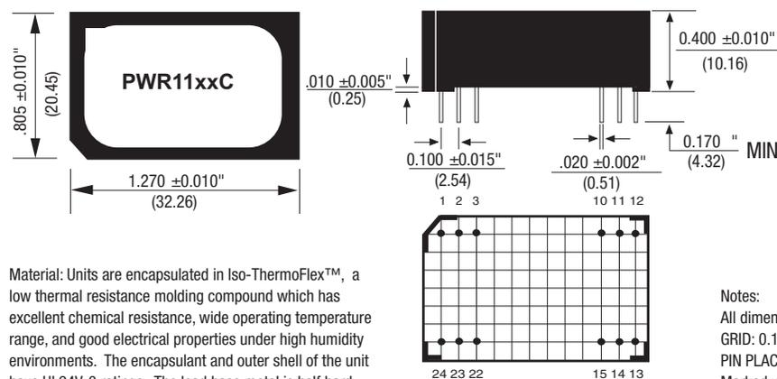
Material: Units are encapsulated in Iso-ThermoFlex™, a low thermal resistance molding compound which has excellent chemical resistance, wide operating temperature range, and good electrical properties under high humidity environments. The encapsulant and outer shell of the unit have UL94V-0 ratings. The lead base metal is half hard brass. Lead finish is matte tin 100 microinches minimum over nickel 40-80 microinches.
