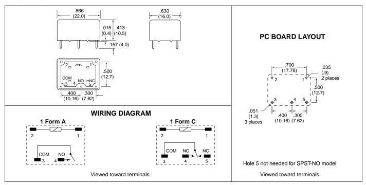
Dimensions in inches with metric equivalents in parentheses. Tolerance: ±0.010"
