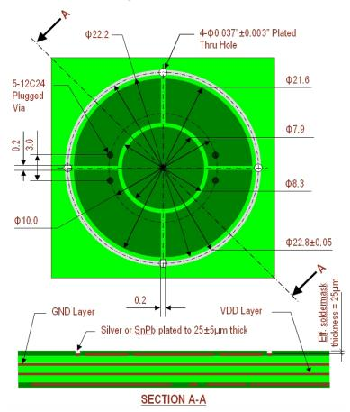
All units are in mm unless specified All tolerances are  $\pm 0.05$  unless specified PCB configurations:-
