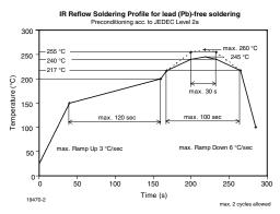
Figure 13. Vishay Lead (Pb) -free Reflow Soldering Profile (acc. to J-STD-020B)
