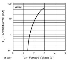
Figure 5. Forward Current vs. Forward Voltage
