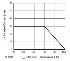
Figure 2. Forward Current vs. Ambient Temperature
