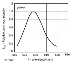
Figure 9. Relative Luminous Intensity vs. Wavelength
