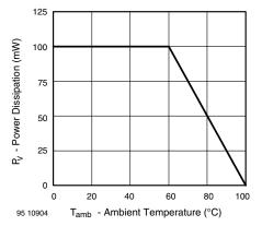
Figure 1. Power Dissipation vs. Ambient Temperature
