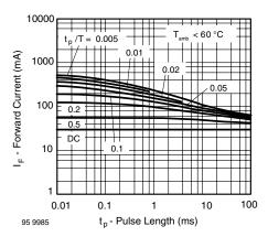
Figure 3. Forward Current vs. Pulse Length
