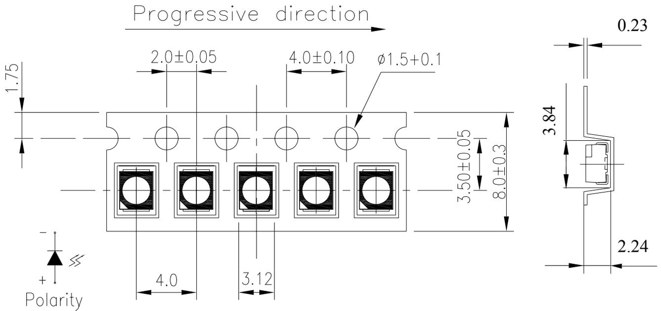
Note: The tolerances unless mentioned is ±0.1mm Unit = mm
