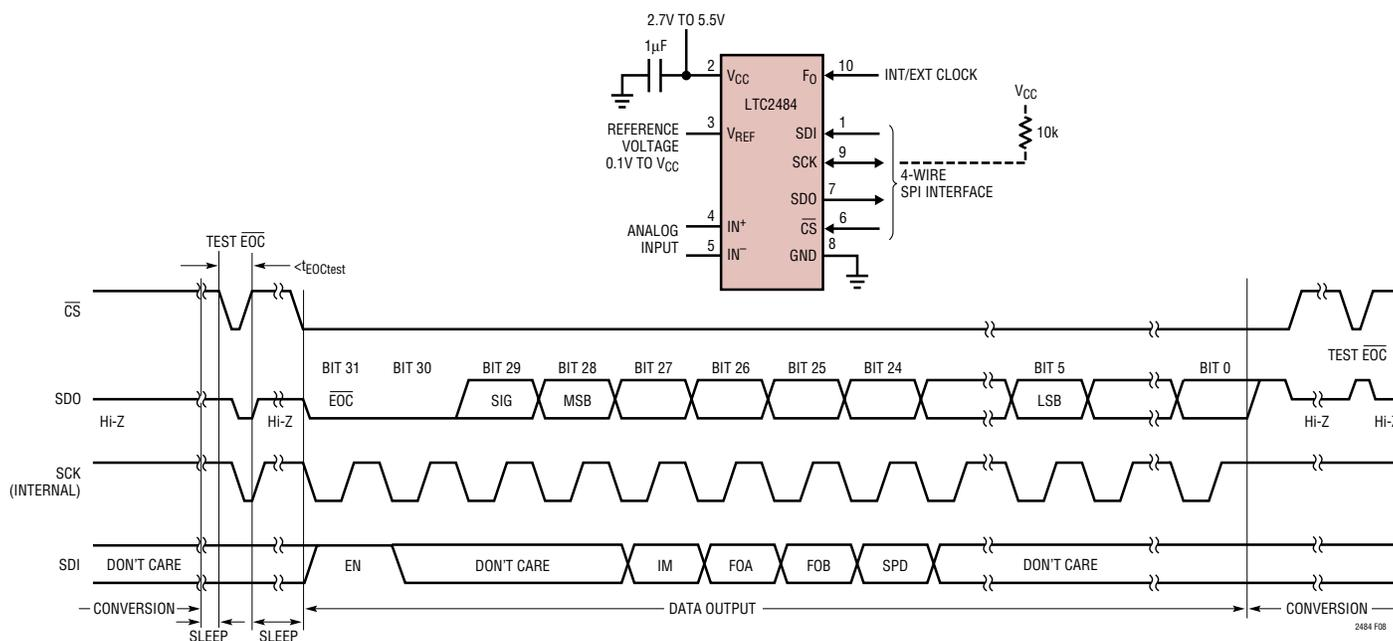
Figure 8. Internal Serial Clock, Single Cycle Operation
