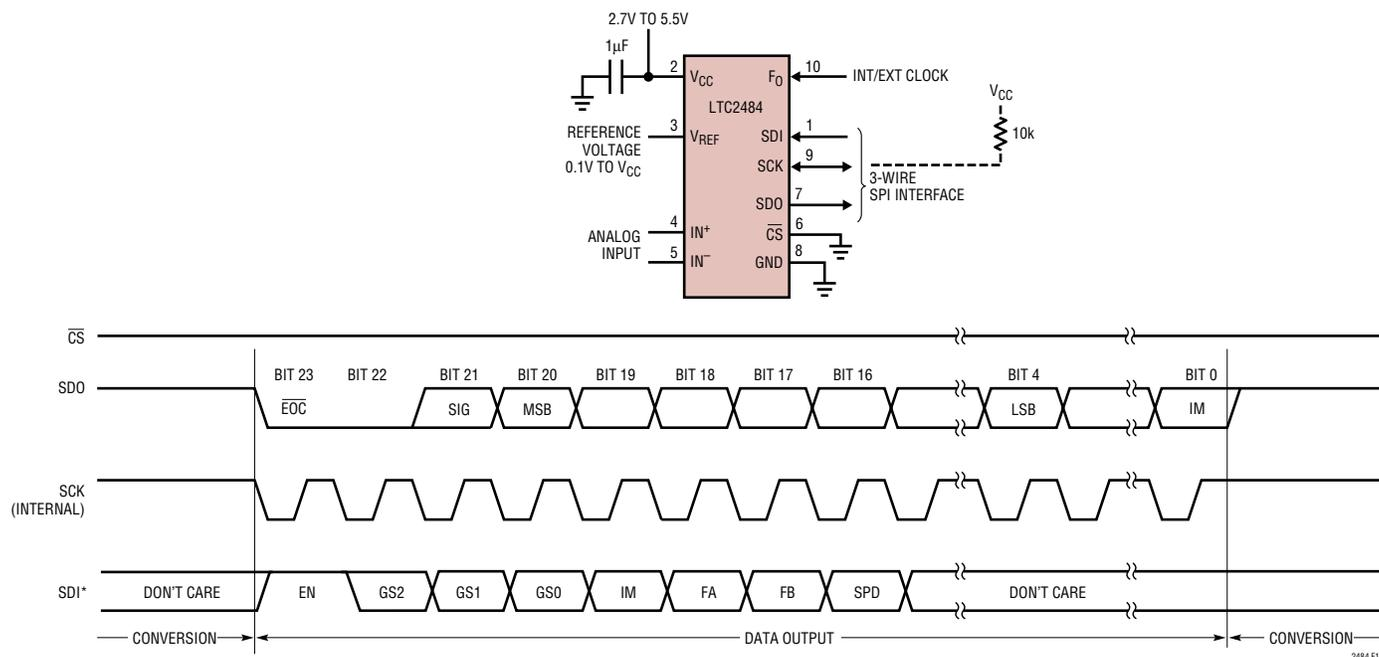
Figure 10. Internal Serial Clock,  $\overline{CS} = 0$  Continuous Operation
