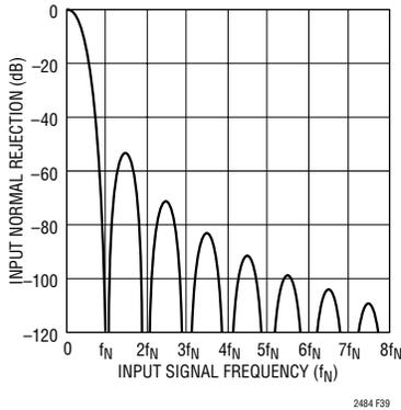
Figure 39. Input Normal Mode Rejection 2x Speed Mode
