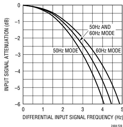
Figure 28. Input Signal Bandwidth Using the Internal Oscillator
