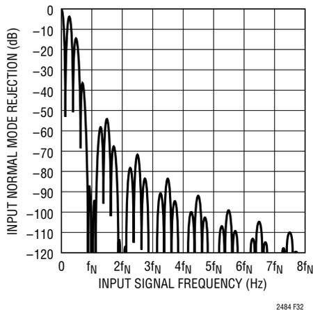
Figure 32. Input Normal Mode Rejection at DC
