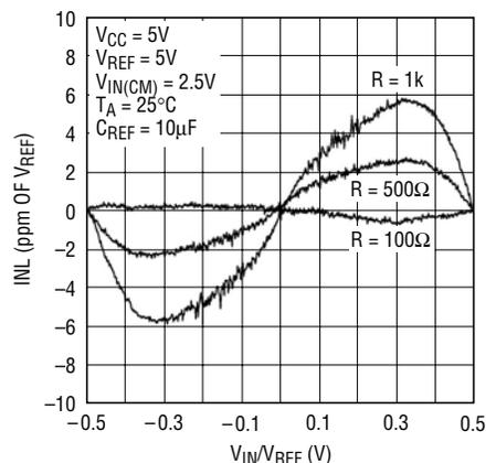
Figure 19. INL vs Differential Input Voltage and Reference Source Resistance for C<sub>REF</sub> > 1μF
