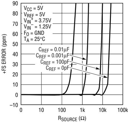
Figure 15. +FS Error vs R<sub>SOURCE</sub> at V<sub>REF</sub> (Small C<sub>REF</sub>)
