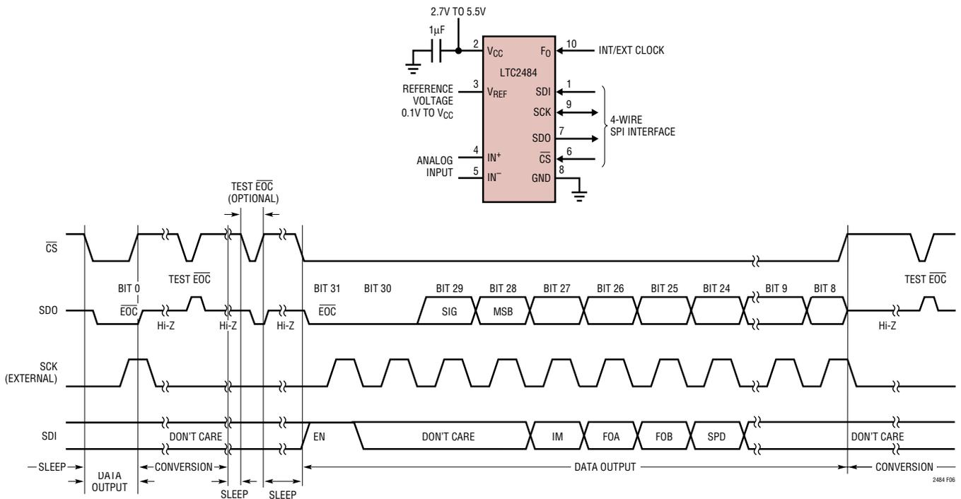
Figure 6. External Serial Clock, Reduced Data Output Length
