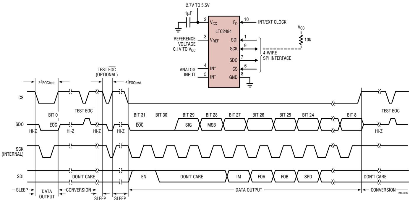
Figure 9. Internal Serial Clock, Reduce Data Output Length
