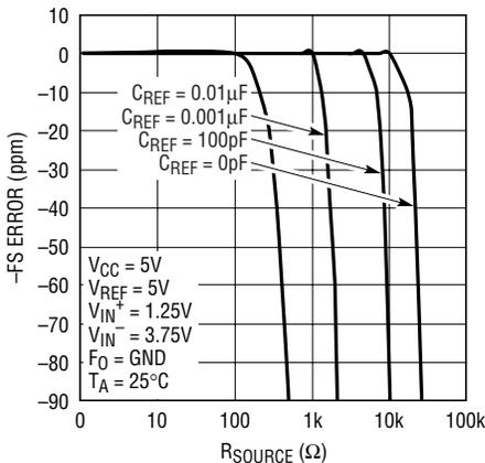
Figure 16. -FS Error vs R<sub>SOURCE</sub> at V<sub>REF</sub> (Small C<sub>REF</sub>)
