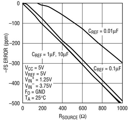
Figure 18. -FS Error vs R<sub>SOURCE</sub> at V<sub>REF</sub> (Large C<sub>REF</sub>)
