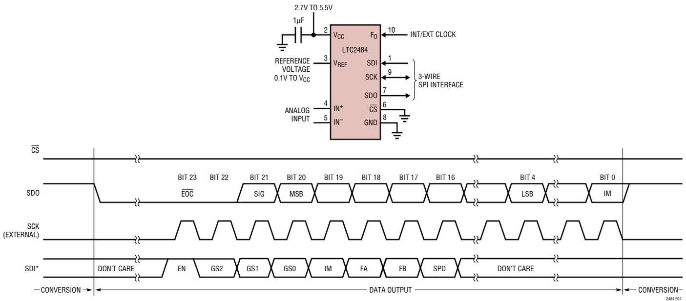
Figure 7. External Serial Clock,  $\overline{CS} = 0$  Operation
