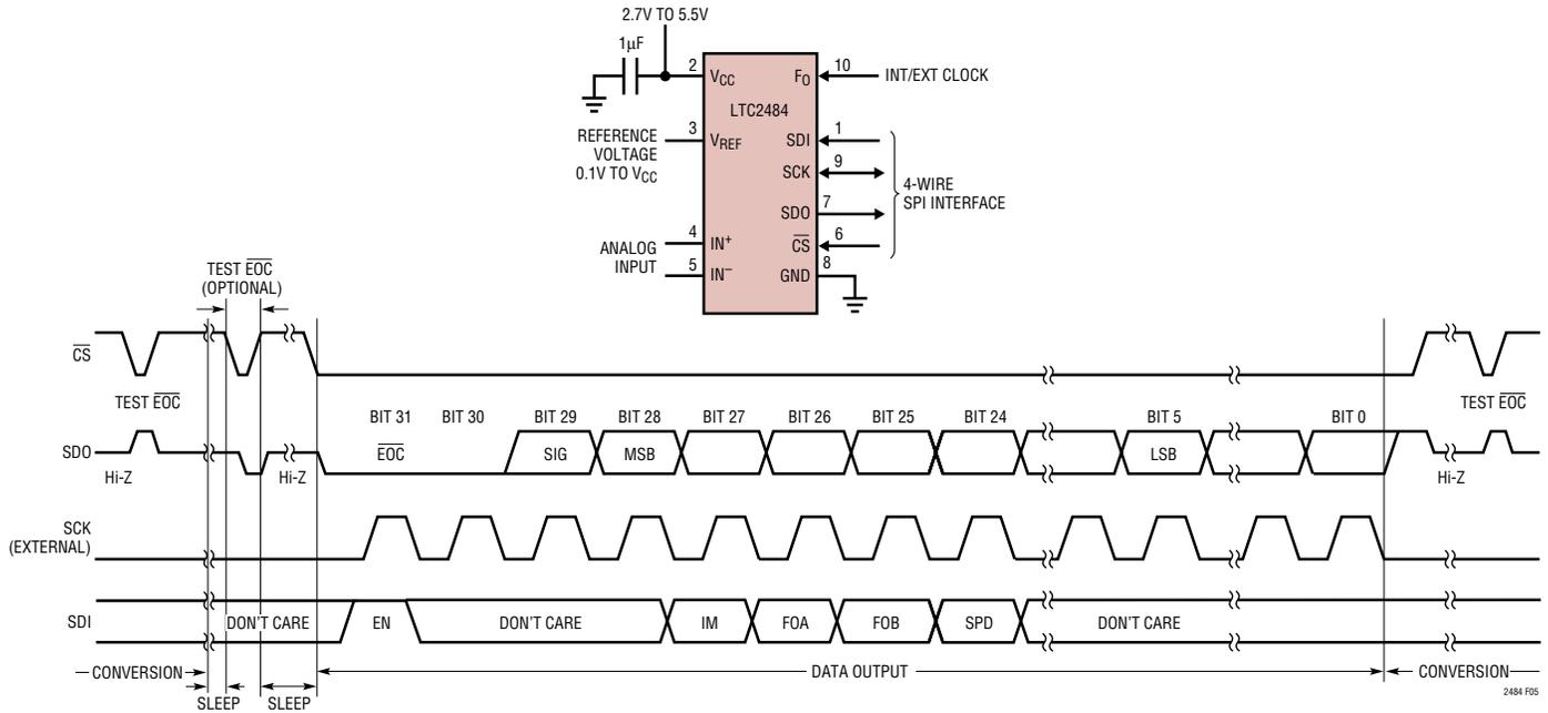
Figure 5. External Serial Clock, Single Cycle Operation
