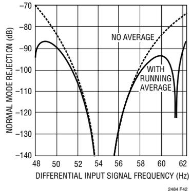
Figure 42. Input Normal Mode Rejection 2x Speed Mode
