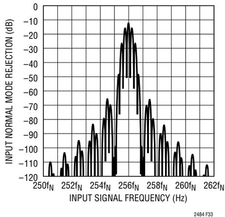
Figure 33. Input Normal Mode Rejection at  $f_S = 256f_N$
