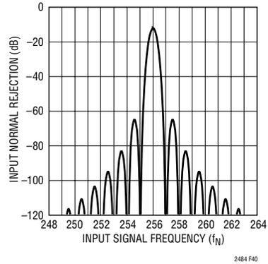
Figure 40. Input Normal Mode Rejection 2x Speed Mode
