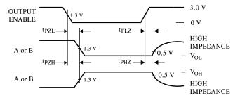
$\begin{array}{l} t_{PZL} \text{ - } S1 \text{ closed, } S2 \text{ opened} \\ t_{PZH^-} S1 \text{ opened, } S2 \text{ closed} \\ t_{PLZ}, t_{PHZ} \text{ - } S1 \text{ and } S2 \text{ closed} \end{array}$
