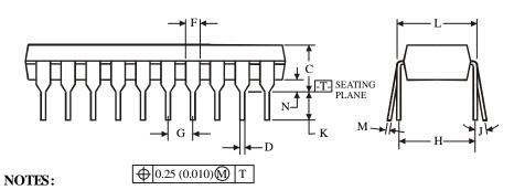
1. Dimensions "A", "B" do not include mold flash or protrusions.
