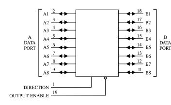
$PIN 20=V_{CC}$  PIN 10 = GND
