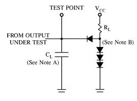
NOTES A.  $C_L$  includes probe and jig capacitance. B. All diodes are 1N916 or 1N3064.
