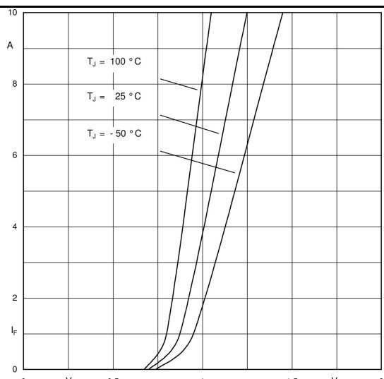
Fig. 1 Forward characteristics (typical values)
