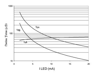
Figure 7. Typical Delay Times
