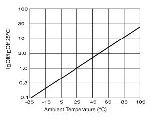
Figure 5. Typical Normalized Off-State Leakage
