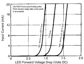
Figure 6. Input Characteristics (Current Controlled)
