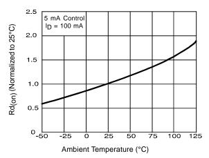
Figure 3.Typical On Characteristics
