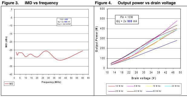
Figure 4. Output power vs drain voltage
