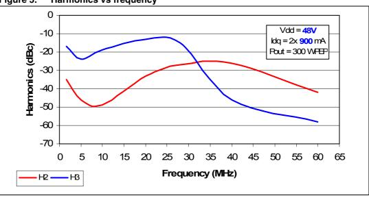
Figure 5. Harmonics vs frequency
