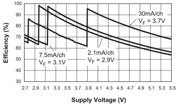
**Flash Efficiency vs. Supply Voltage**
