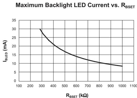
**Figure 3: Maximum LED Current vs R<sub>BSET</sub>.**
