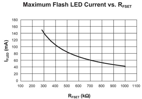
**Figure 4: Maximum Flash Current vs. R<sub>FSET</sub>.**
