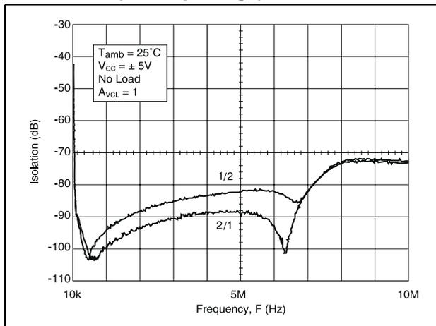
**Figure 11. Cross talk isolation vs. frequency (SO-14 package)**
