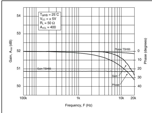
**Figure 9. Gain flatness & phase shift vs. frequency**
