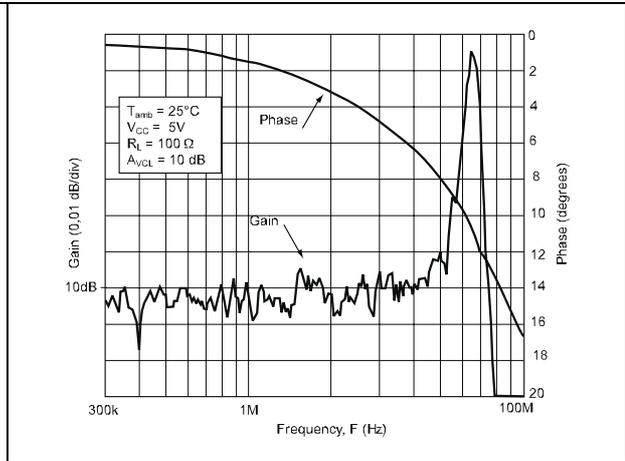
**Figure 10. Cross talk isolation vs. frequency (SO-14 package)**
