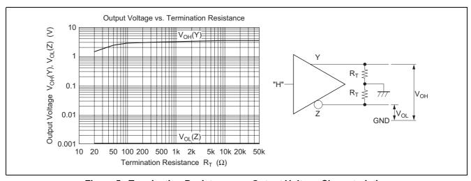
Figure 5 Termination Resistance vs. Output Voltage Characteristics
