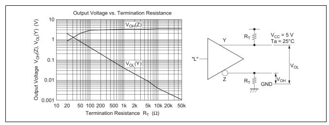
Figure 8 Termination Resistance vs. Output Voltage Characteristics
