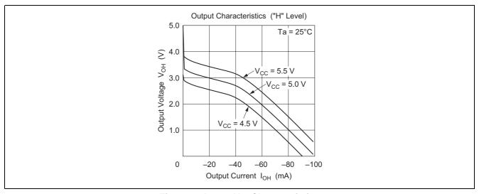
Figure 1 I<sub>OH</sub> vs. V<sub>OH</sub> Characteristics
