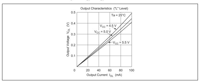
Figure 2 I<sub>OL</sub> vs. V<sub>OL</sub> Characteristics
