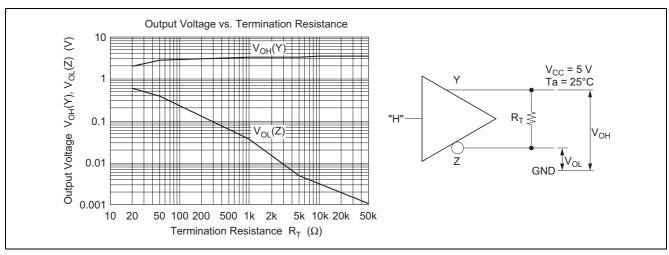
Figure 6 Termination Resistance vs. Output Voltage Characteristics
