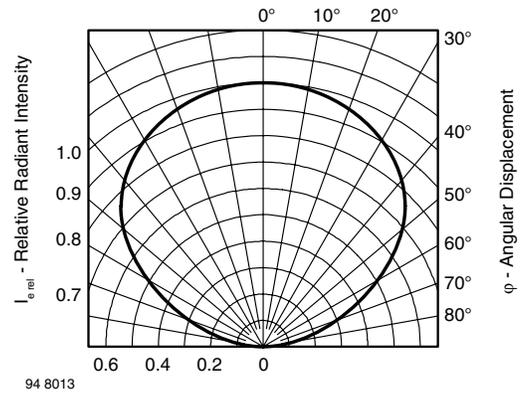
Fig. 7 - Relative Radiant Intensity vs. Angular Displacement
