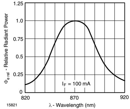
Fig. 6 - Relative Radiant Power vs. Wavelength
