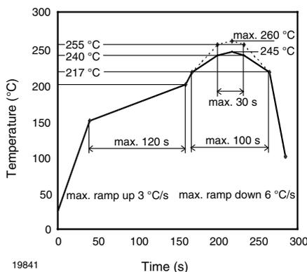
Fig. 8 - Lead (Pb)-free Reflow Solder Profile acc. J-STD-020D
