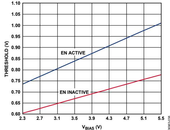
Figure 38. Typical EN Pin Thresholds vs. Input
