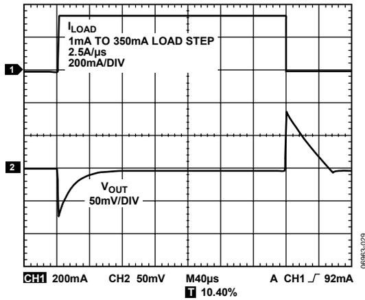
Figure 29. Load Transient Response
