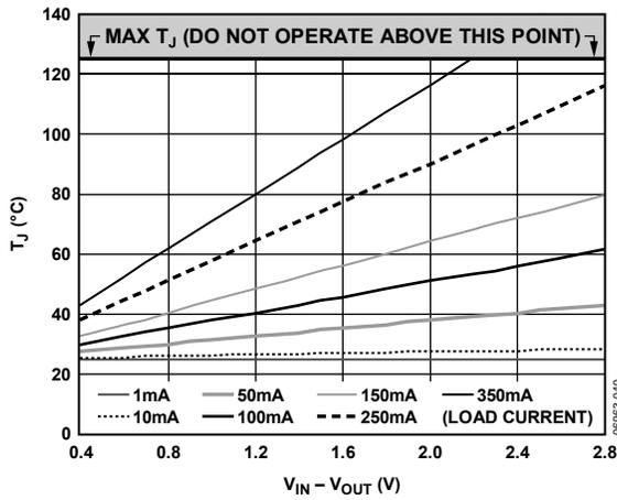
Figure 40. 500 mm<sup>2</sup> of PCB Copper, T<sub>A</sub> = 25°C, TSOT
