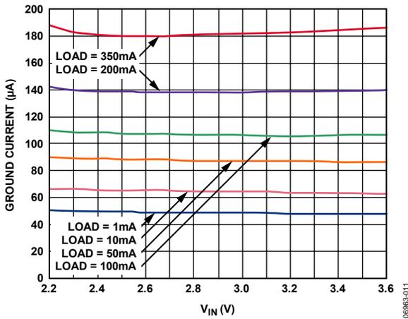
Figure 11. Ground Current vs. Input Voltage
