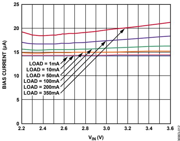
Figure 12. Bias Current vs. Input Voltage
