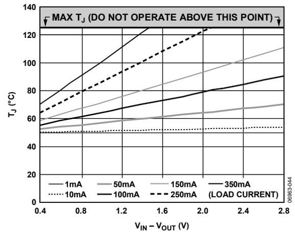
Figure 44. 100 mm<sup>2</sup> of PCB Copper, T<sub>A</sub> = 50°C, TSOT
