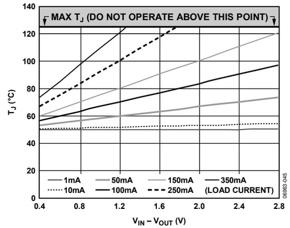
Figure 45. 0 mm<sup>2</sup> of PCB Copper, T<sub>A</sub> = 50°C, TSOT
