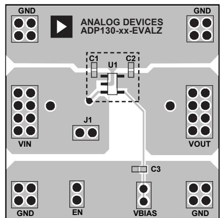
Figure 47. Example TSOT PCB Layout
