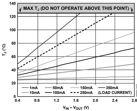
Figure 42. 0 mm<sup>2</sup> of PCB Copper, T<sub>A</sub> = 25°C, TSOT
