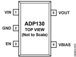
Figure 3. Pin Configuration
