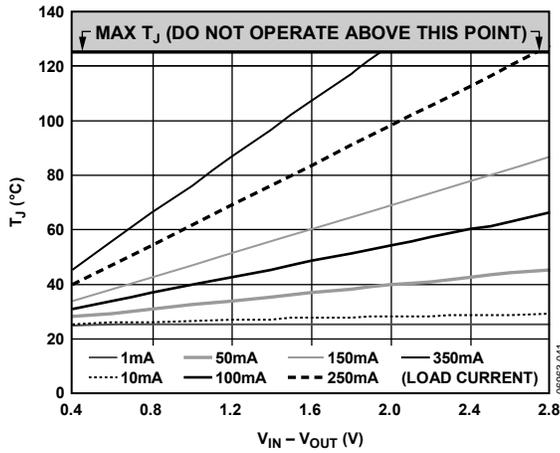
Figure 41. 100 mm<sup>2</sup> of PCB Copper, T<sub>A</sub> = 25°C, TSOT
