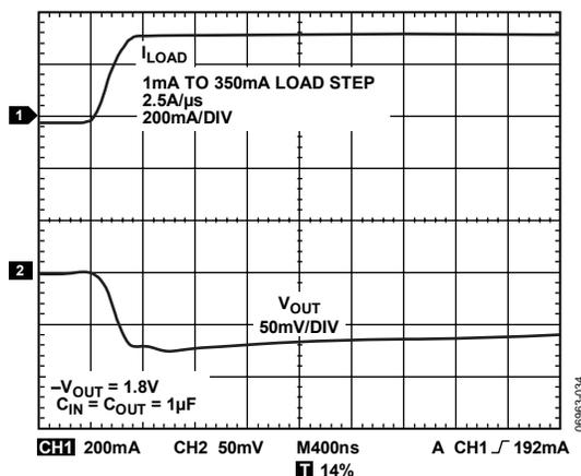
Figure 34. Output Transient Response,  $C_{OUT} = 1\ \mu\text{F}$
