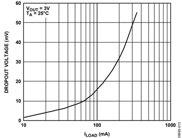
Figure 13. Dropout Voltage vs. Load Current,  $V_{OUT} = 3V$
