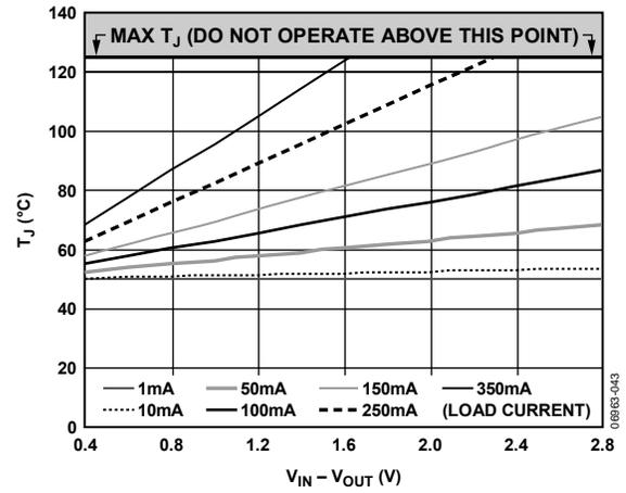
Figure 43. 500 mm<sup>2</sup> of PCB Copper, T<sub>A</sub> = 50°C, TSOT
