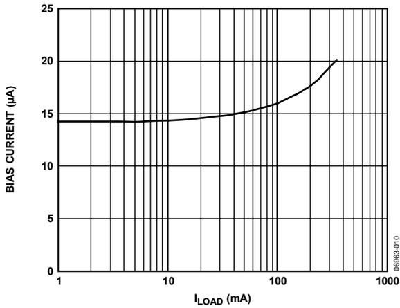
Figure 10. Bias Current vs. Load Current
