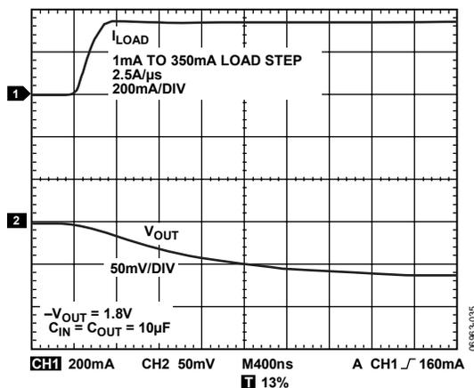
Figure 35. Output Transient Response,  $C_{OUT} = 10\ \mu\text{F}$
