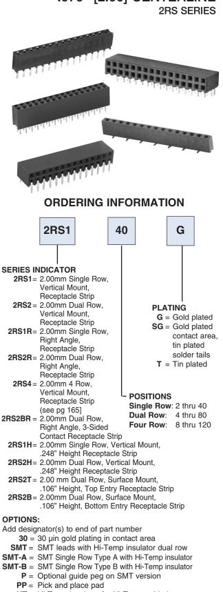
**HT** = Hi-Temp insulator for Hi-Temp soldering processes up to 260°C (*Add this option for thru-hole products only. All SMT products are manufactured with Hi-Temp insulators*)
