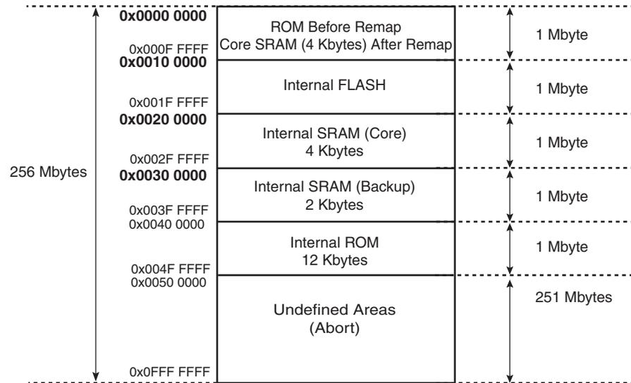
**Figure 8-3.** Internal Memory Mapping with GPNVM Bit 1 = 1
