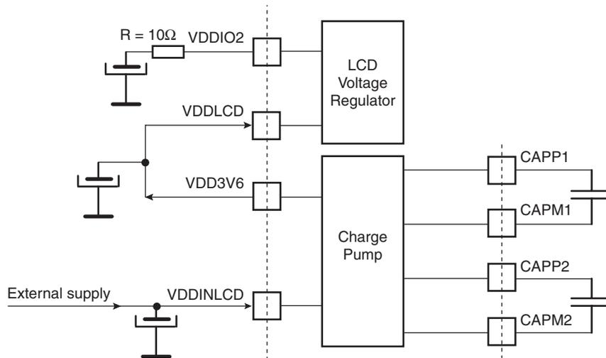
**Figure 5-4.** The LCD Regulator is Externally Supplied
