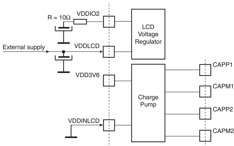
If the charge pump is not needed, the user can apply an external voltage. See [Figure 5-5](#) below:
