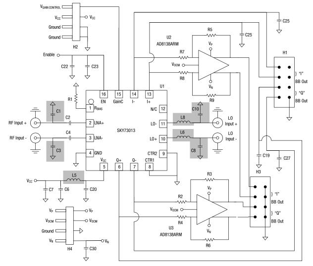
C1, C3, C8, C10 not installed. Zero  $\Omega$  resistors installed in positions L5, L6, and L8. U2, U3, and associated components are installed to facilitate nosie figure measurements.
