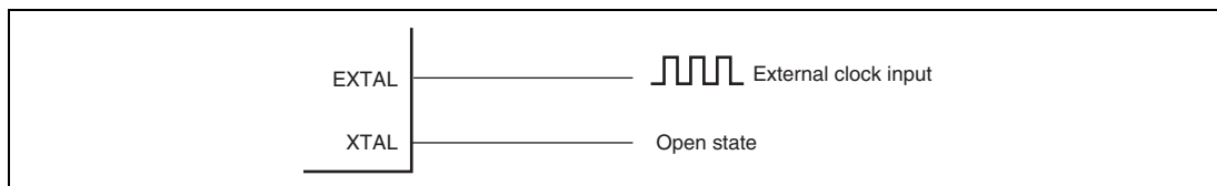
Figure 4.4 Example of External Clock Connection
