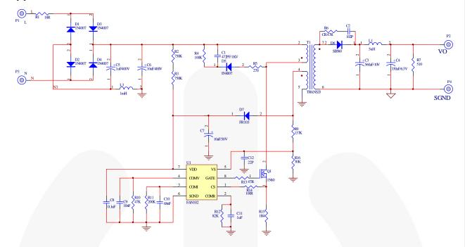
Figure 26. 5W (5V/1A) Application Circuit
