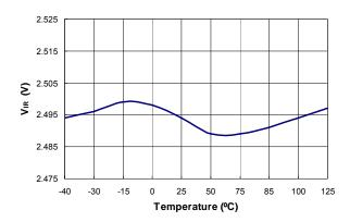
Figure 10. Reference Voltage (V<sub>VR</sub>) vs. Temperature
