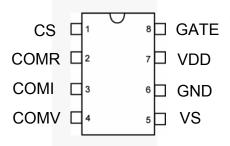
Figure 5. Pin Configuration
