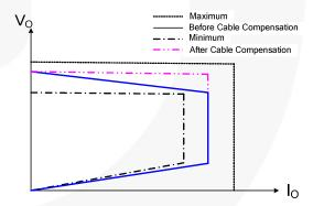
Figure 1. Typical Output V-I Characteristic
