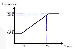
Figure 25. Green Mode Frequency vs. V<sub>COMV</sub>
