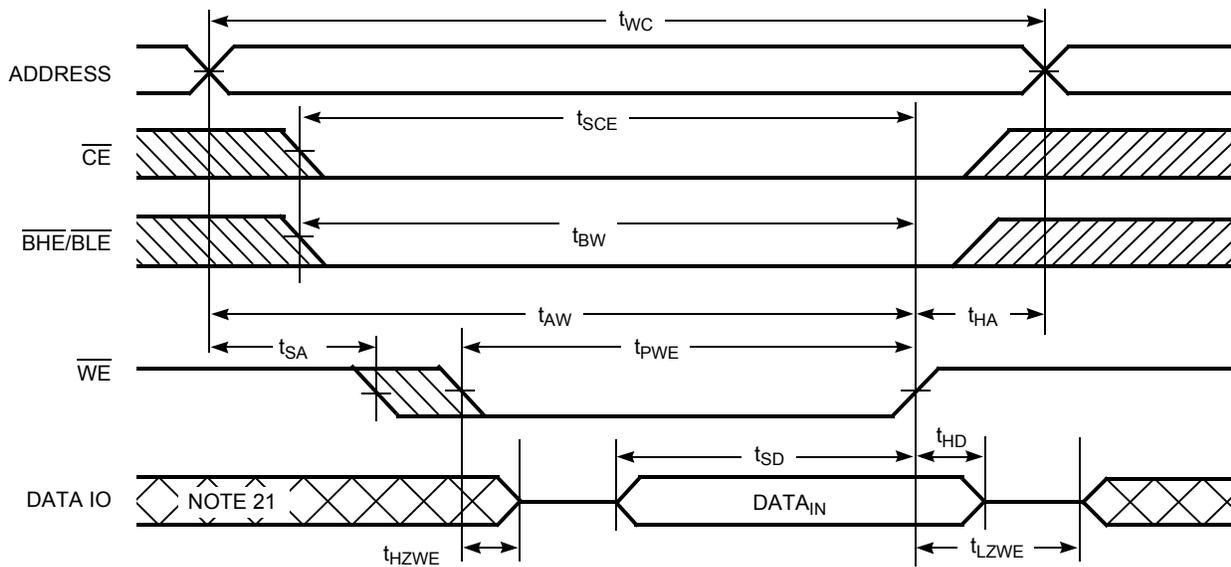
Figure 10. Write Cycle 4:  $\overline{BHE/BLE}$  Controlled,  $\overline{OE}$  LOW [20]
