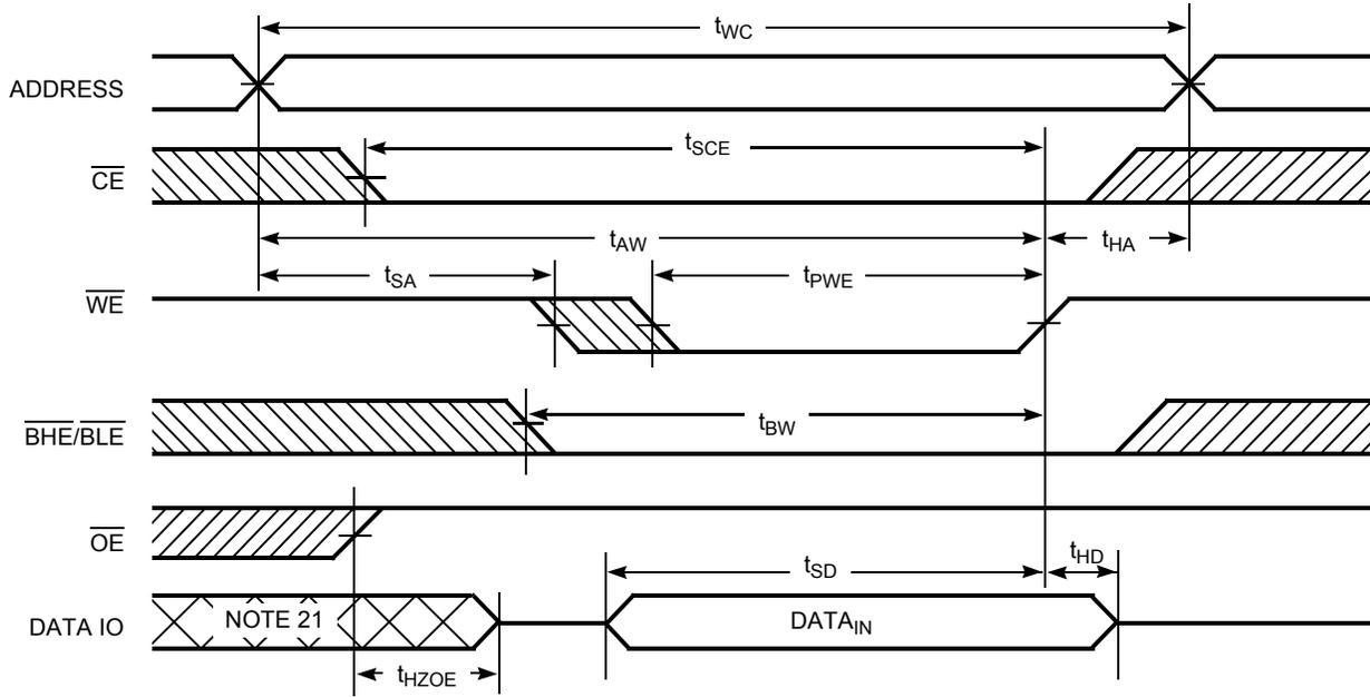
Figure 8. Write Cycle 2:  $\overline{CE}$  Controlled [15, 19, 20]
