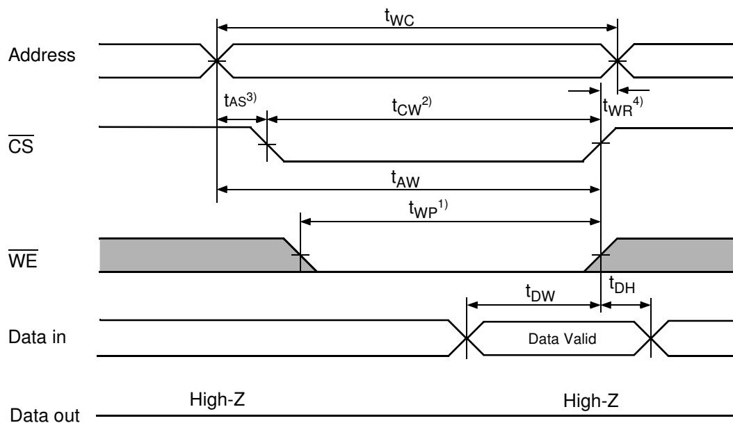
**TIMING WAVEFORM OF WRITE CYCLE(3) ( $\overline{\text{WE}}$  Controlled,  $\overline{\text{OE}}$  LOW)**
