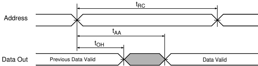
**TIMING WAVEFORM OF READ CYCLE(2) ( $\overline{OE}$  Controlled)**
