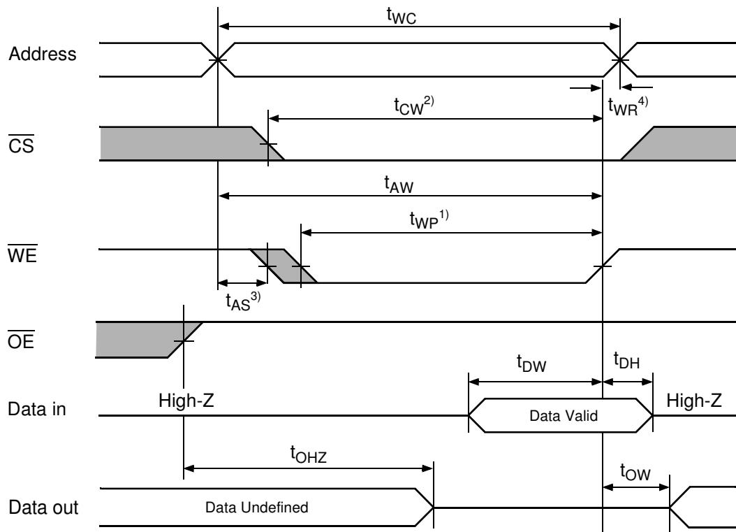
**TIMING WAVEFORM OF WRITE CYCLE(2) ( $\overline{\text{CS}}$  Controlled)**
