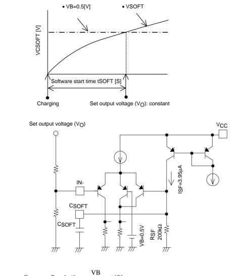
$t_{\text{SOFT}} = -C_{\text{SOFT}} \times R_{\text{SF}} \ln(1 - \frac{\text{VB}}{R_{\text{SF}} \times I_{\text{SF}}})[S]$
