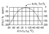
The curve shown above accounts for resonator contribution only and does not include oscillator temperature characteristics.
