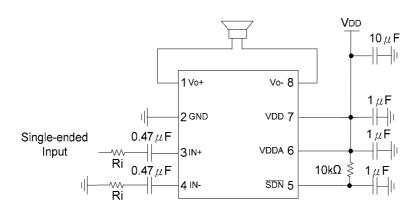
Figure.2 Single-ended Input With Gain= 320k 15k+Ri
