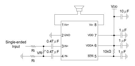
Figure.5 Single-ended Input With Gain Control
