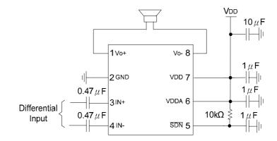
Suppose source impedance of the input is much smaller than 15k.
