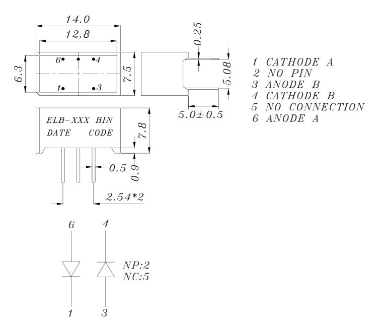
**Notes:** 1.All dimensions are in millimeters , tolerance is 0.25mm unless otherwise noted.
