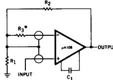
$$\text{NOTE: } \frac{R_1 R_2}{R_1 + R_2} \text{ Must be low impedance}$$
