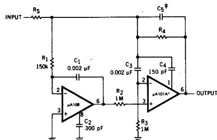
\*In addition to increasing speed, the 101A raises high and low frequency gain, increases output drive capability and eliminates thermal feedback.
