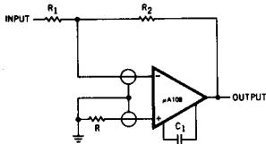
$$R = \frac{R_1 R_2}{R_1 + R_2}$$
