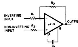
$$C_f \geq 30 \left( \frac{1}{1 + \frac{R_2}{R_1}} \right)$$
