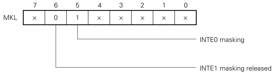
Figure 6-25. Interrupt Mask Register (MKL) Setting (Single Pulse Output: INTE1 Mask Release)
