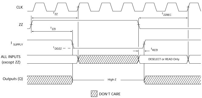
21. Device must be deselected when entering ZZ mode. See Cycle Descriptions table for all possible signal conditions to deselect the device. 22. I/Os are in High-Z when exiting ZZ sleep mode.
